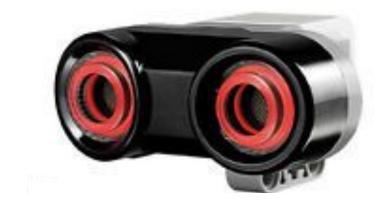
We can use the ultrasonic sensor to stop at a number of centimeters away from something almost like stopping at a color. Create a regular stop at a color program. Then change the setting of the wait block to "Ultrasonic Sensor", "Compare", "Distance Centimeters". Change the number of centimeters to 20, and make the compare setting "Less than or equal to"
