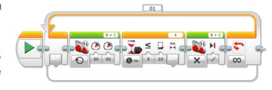
Then in the loop (after the move to distance program), program the robot to move back and turn 0.7 rotations. This code will keep moving forward until the robot is close to something, and then move back and turn around so that it doesn't hit it.
